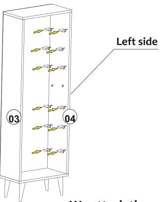
We attach the rack pins to parts 3 and 4
