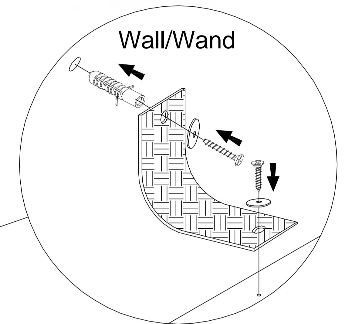
**⚠ Warning:** To keep safety, the cabinet has to be fixed to a wall with the anti-tipping accessories which are supplied.
